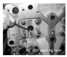
Loctite® RC™ 620 is applied in a bead to the upper end of the injector tubes (top), and the interior of the engine housing (bottom) prior to installation. RC 620 has helped increase the life of the rebuilt Komatsu engines due to its high temperature performance and its high chemical resistance.
